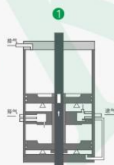
1 开阀初始阶段工作力=2P Initial operating force of valve opening = 2P
